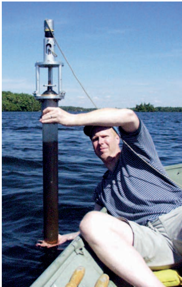
Figure 2 Retrieving surface sediment cores with a Glew gravity corer from Lake Opinicon (Canada). Photograph courtesy of B. Cumming (Queen's University).
