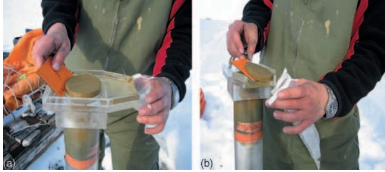
Figure 3 An example of a vertical extrusion system used for sectioning recent sediment at close intervals. (a) A 1 cm slice of sediment has been extruded from the core tube. (b) The sediment section is sliced off and removed. Photographs courtesy of N. Michelutti (Queen's University).
