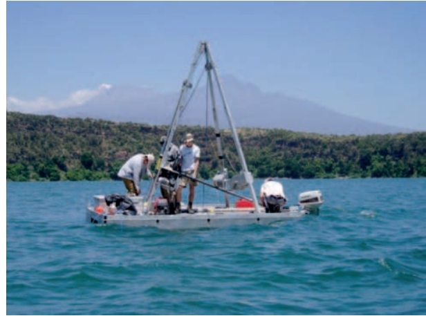
Figure 1 Lake sediment coring on Lake Chala (Kenya), using a Livingstone-type piston corer (modified by UWITEC). Photograph courtesy of B. Cumming (Queen's University).
